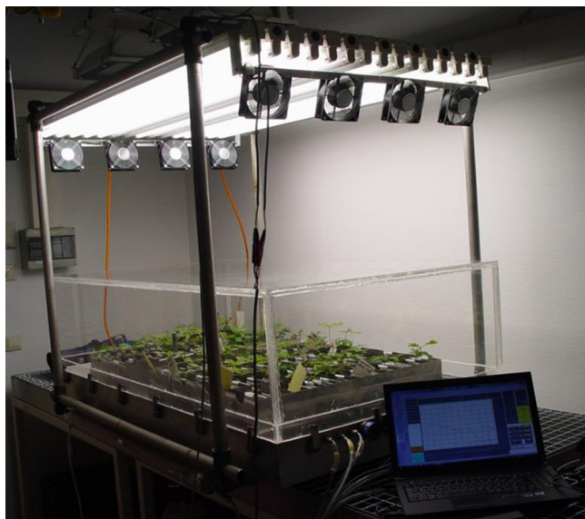
Fig. 5. Plexiglas chamber used to label the oak microcosms with ^{13}\text{C} (see Appendix 2 of Supporting information).
